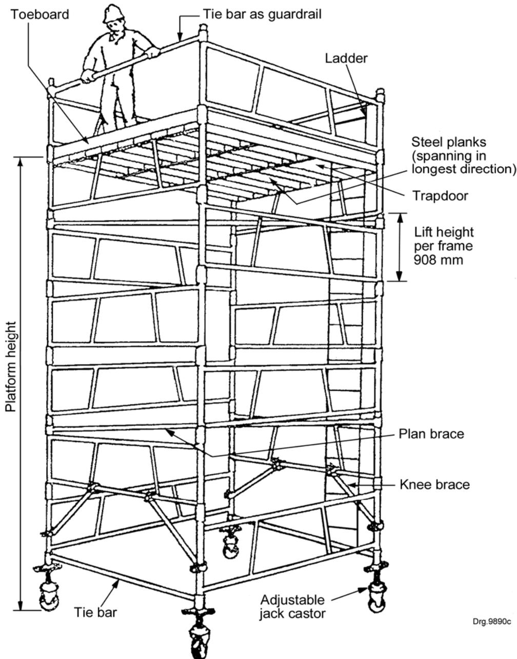
**Figure 1 — Tubular steel mobile tower (interlocking frame scaffolding)**
